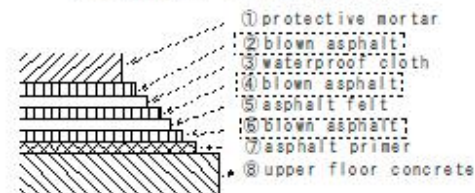
An example of top waterproofing
