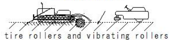
Lime stabilization method Lime/quicklime
